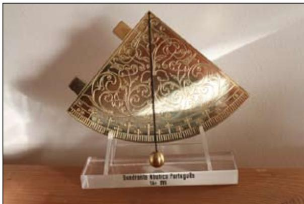
*Figure 1. Portuguese Mariners Quadrant (Quarter of a Circle) showing sighting pin holes and plumb line.*
